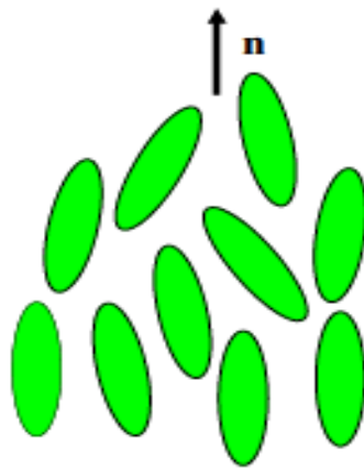
Figure 1. 5. Schematic representation of the molecular organization in the N phase of the calamitic LCs
